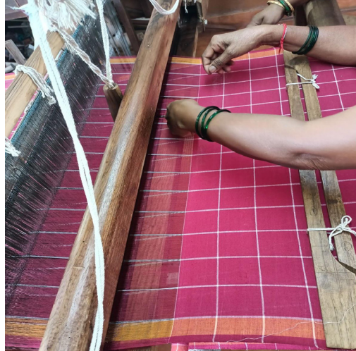
Figure 11: weaving on the loom. (sari without the doobby border)
