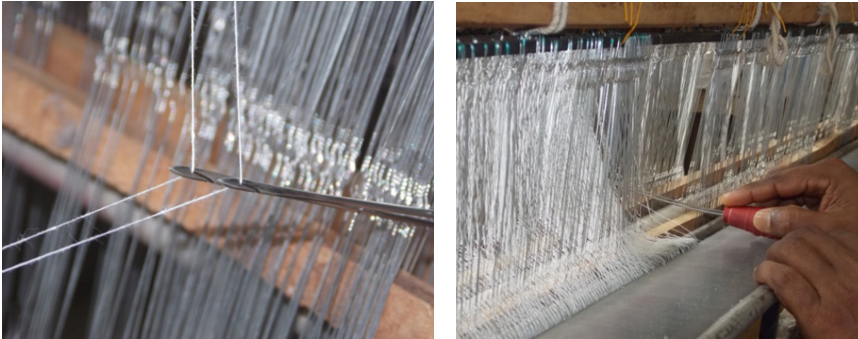
Figure 8: Denting in & drawing operation.
