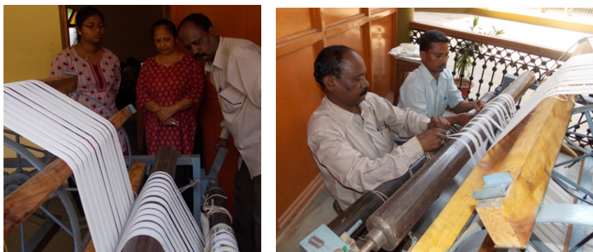
Figure 10: Tying the threads to the warp beam.
