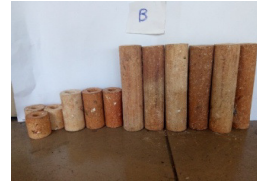
Plate 16: Result of fired Props Recipe B
