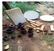
Plate 21: Offloaded glazed wares, shelves and props
