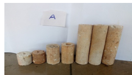
Plate 15 : Result of fired Props Recipe A
