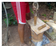
Plaste 11: Extruding the Prop
