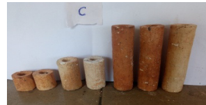
Plate 17: Result of fired Props Recipe C
