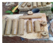
Plaste 13: Drying of Moulded Props
