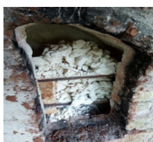
Plate 1: Firing of levigated kaolin using kerosene kiln
