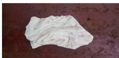
Plate 2: Fired levigated kaolin
