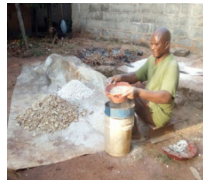
Plate 3: Sieving grog using 80, 100 and 120 mesh
